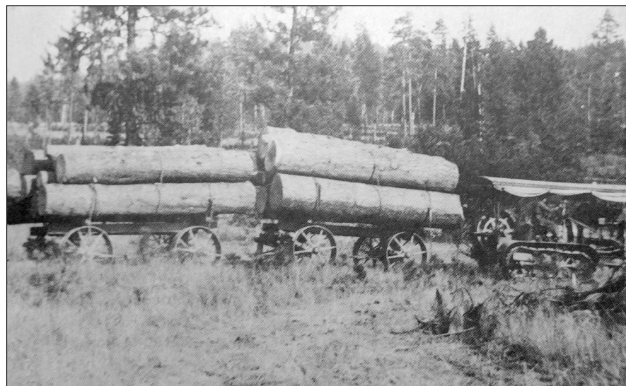
Track-laying tractor hauls up to four wagons of logs to landing in O'Gara Bay for Grant Lumber Co.
